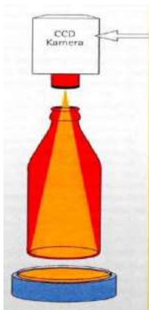
Figure bottom inspection
